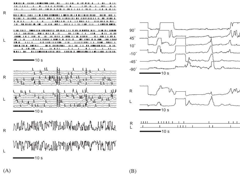
Fig. 2. A closed-loop experiment. (A). From top to bottom: neural activity in the output (motor) areas, estimated instantaneous firing rates and computed angular speeds of the robot wheels. (B). From top to bottom, activity of the robot sensors, rates and corresponding patterns of stimulation.
