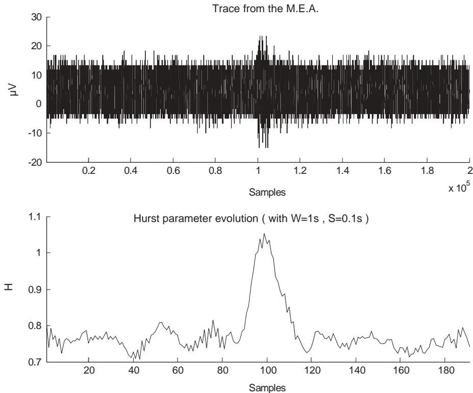
Fig. 1. Evolution of the Hurst parameter in relation to the neural signal from one recording site.
